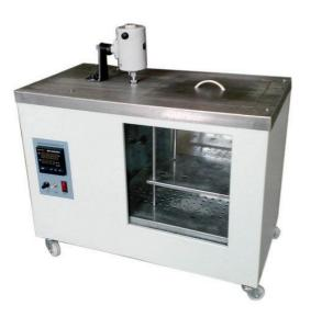
Resistance to environmental stress cracking tester is mainly used to determine the ethylene-based resin and plastic stress cracking ability.
